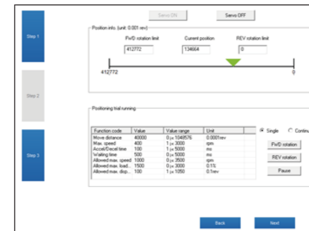
Easy auto-tuning using position JOG and self-adjustment
